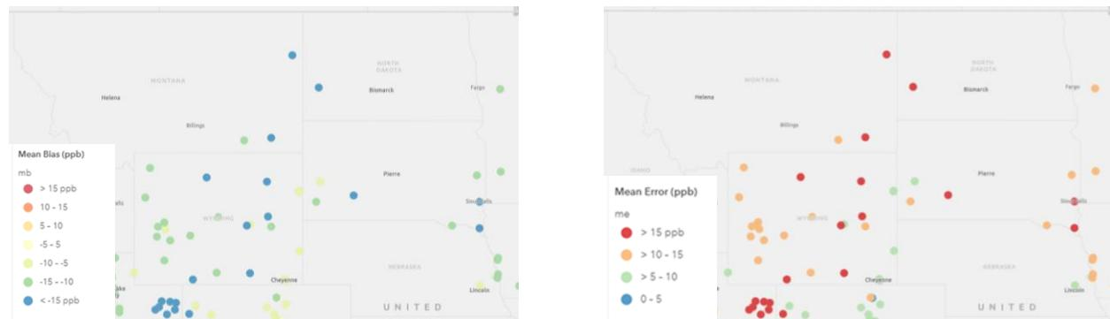
**Figure 49. Mean Bias (ppb) [left] and Mean Error (ppb) [right] of MDA8 ozone  $\geq 60$  ppb over the period May-September 2016 at AQS monitoring sites in West-North-Central region.**
