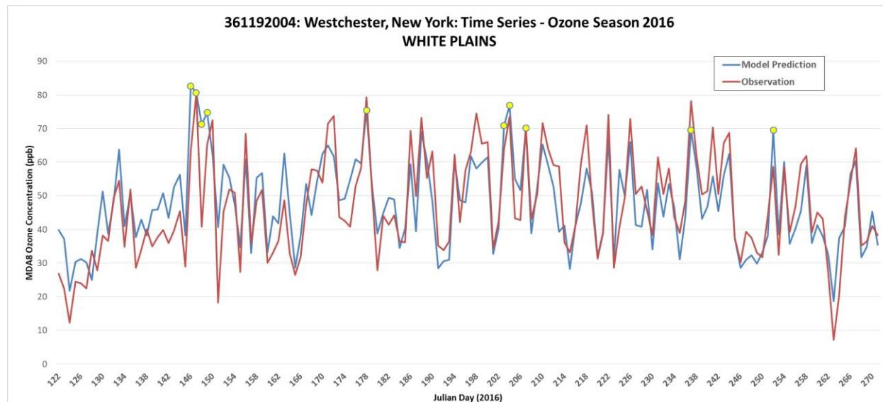
**Figure 94.** Time series of observed (red) and predicted 12km (blue) MDA8 ozone for May through September 2016 at site 361192004. Yellow dots indicate top modeled values.
