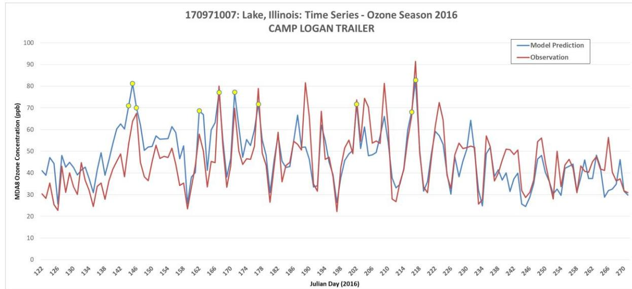
**Figure 70.** Time series of observed (red) and predicted 12km (blue) MDA8 ozone for May through September 2016 at site 170971007. Yellow dots indicate top modeled values.
