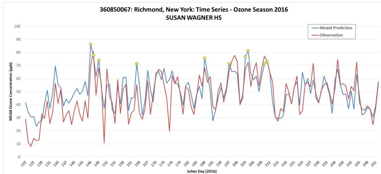
**Figure 92.** Time series of observed (red) and predicted 12km (blue) MDA8 ozone for May through September 2016 at site 360850067. Yellow dots indicate top modeled values.
