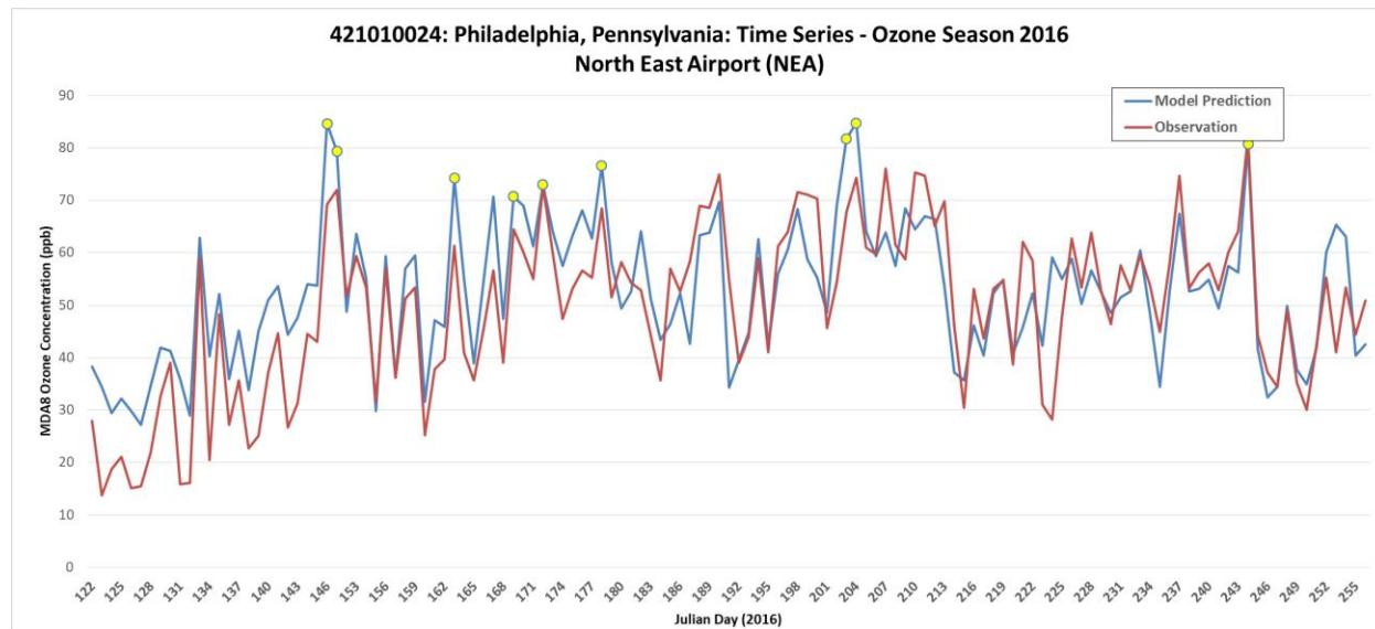
**Figure 98.** Time series of observed (red) and predicted 12km (blue) MDA8 ozone for May through September 2016 at site 421010024. Yellow dots indicate top modeled values.
