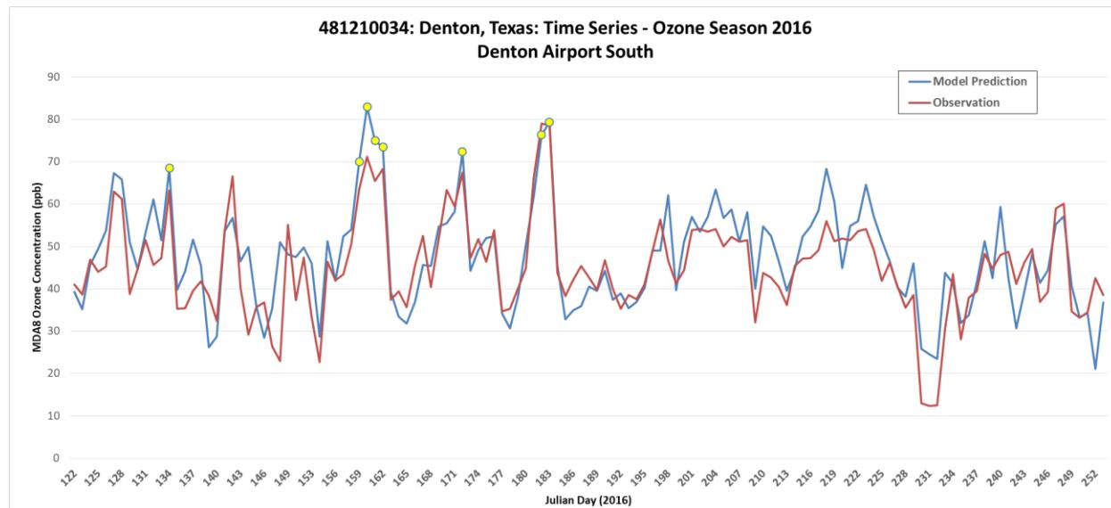
Figure 100. Time series of observed (red) and predicted 12km (blue) MDA8 ozone for May through September 2016 at site 481210034. Yellow dots indicate top modeled values.
