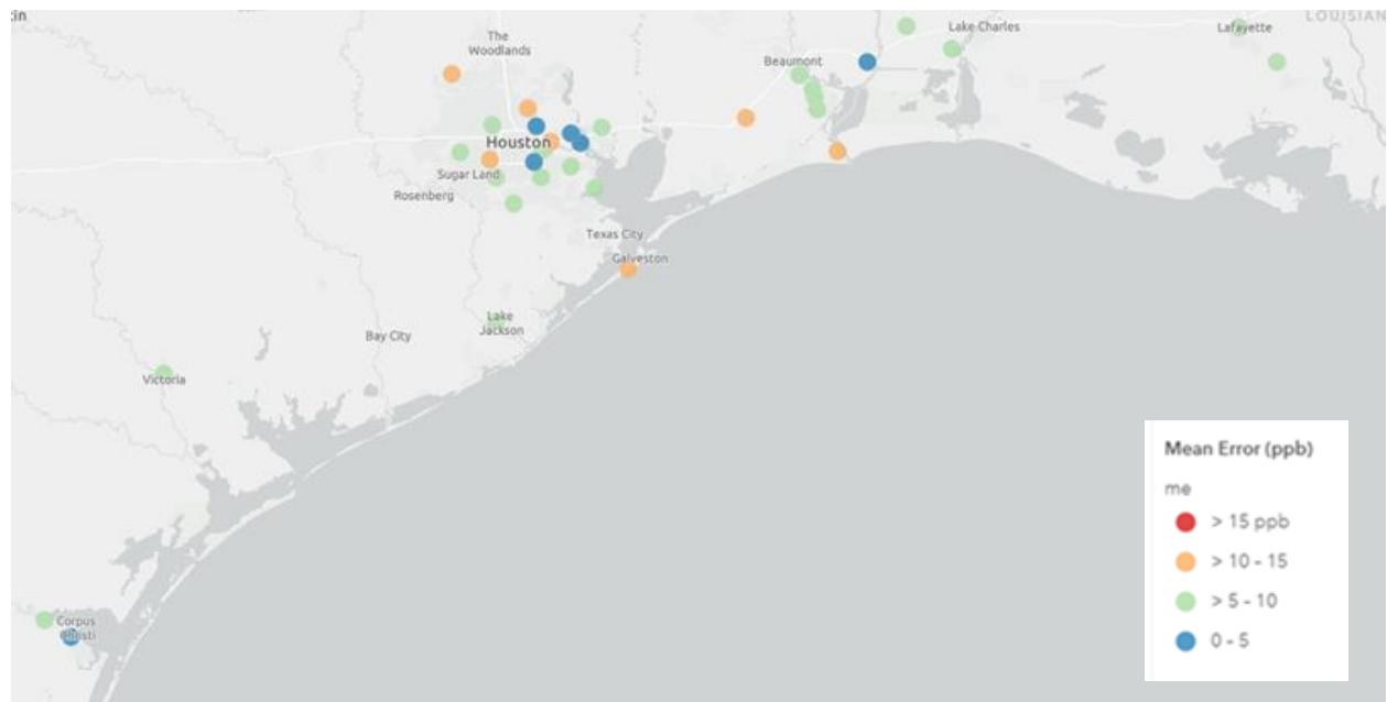
**Figure 56. Mean Error (ppb) of MDA8 ozone  $\geq 60$  ppb over the period May-September 2016 at AQS monitoring sites in Gulf Coast region.**
