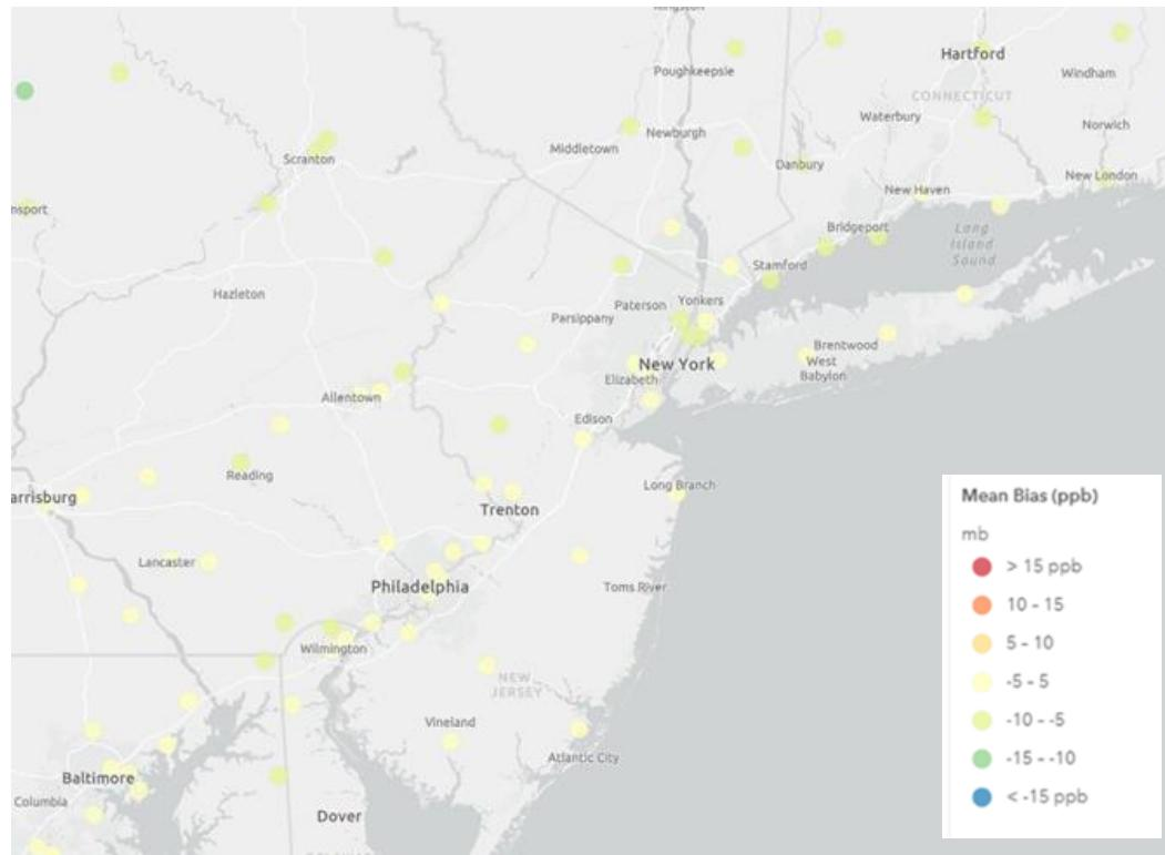
**Figure 63. Mean Bias (ppb) of MDA8 ozone  $\geq 60$  ppb over the period May-September 2016 at AQS monitoring sites in I-95 region.**
