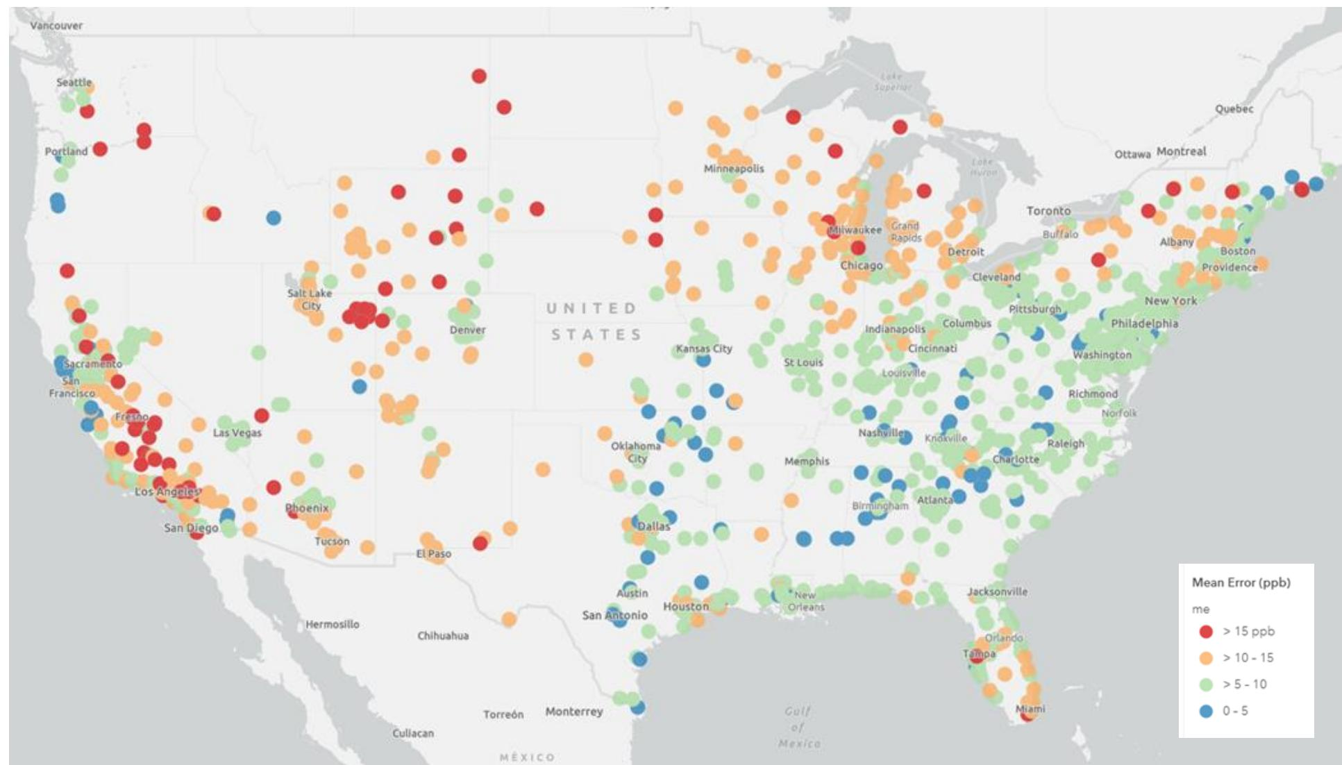
Figure 4. Mean Error (ppb) of MDA8 ozone  $\geq 60$  ppb over the period May-September 2016 at AQS monitoring sites.
