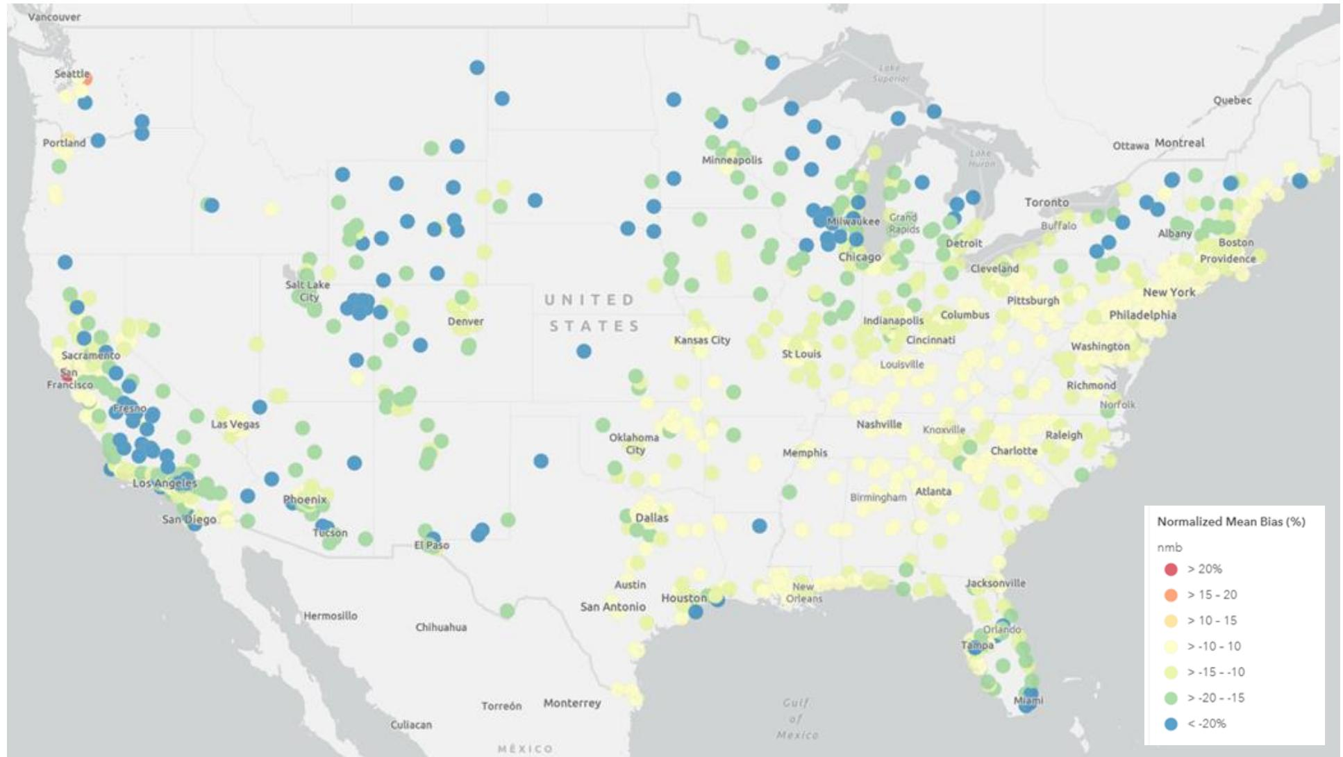
Figure 5. Normalized Mean Bias (%) of MDA8 ozone  $\geq 60$  ppb over the period May-September 2016 at AQS monitoring sites.
