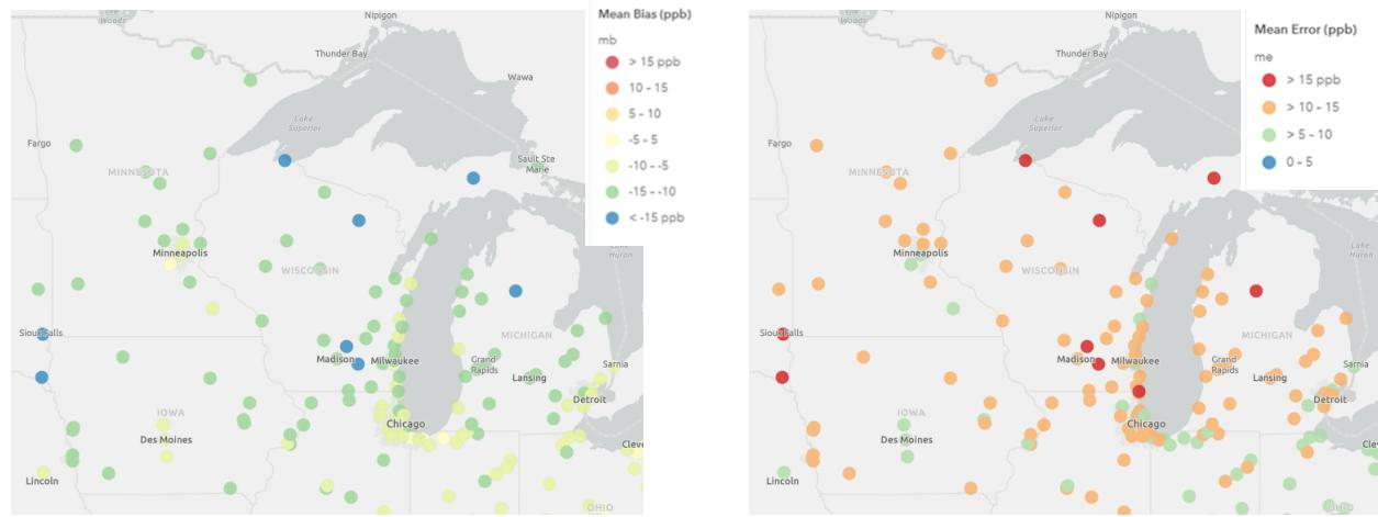
**Figure 14. Mean Bias (ppb) [left] and Mean Error (ppb) [right] of MDA8 ozone  $\geq 60$  ppb over the period May-September 2016 at AQS monitoring sites in East-North-Central region.**
