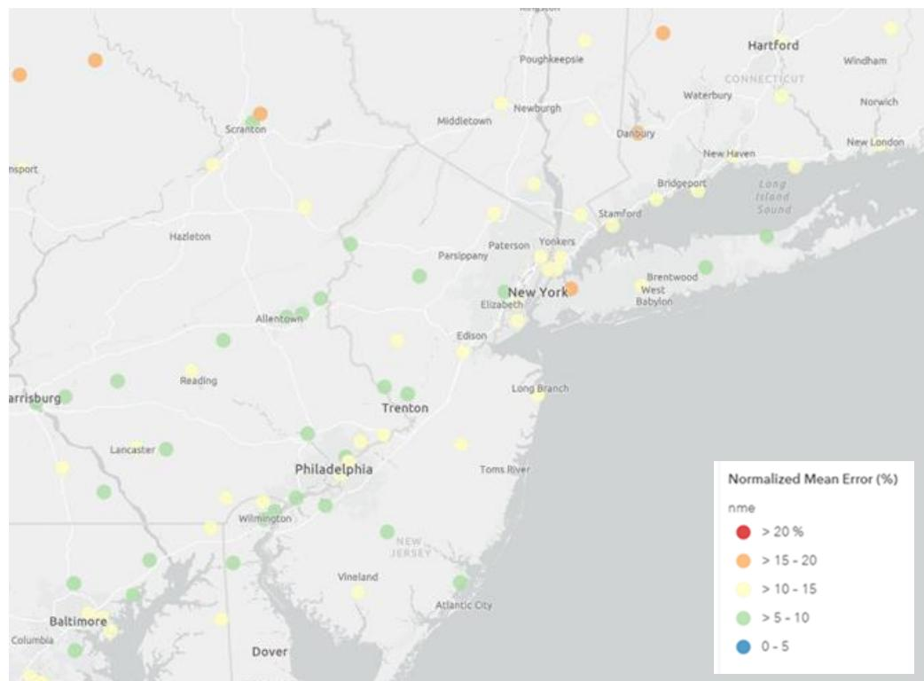
**Figure 66.** Normalized Mean Error (%) of MDA8 ozone  $\geq 60$  ppb over the period May-September 2016 at AQS monitoring sites in I-95 region.
