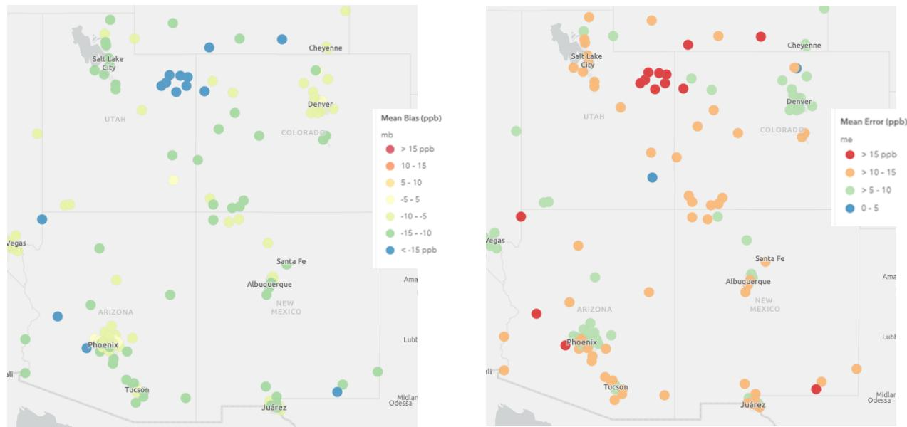
**Figure 39. Mean Bias (ppb) [left] and Mean Error (ppb) [right] of MDA8 ozone  $\geq 60$  ppb over the period May-September 2016 at AQS monitoring sites in Southwest region.**
