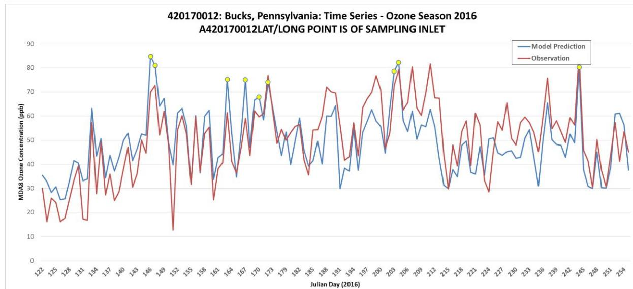
**Figure 96.** Time series of observed (red) and predicted 12km (blue) MDA8 ozone for May through September 2016 at site 420170012. Yellow dots indicate top modeled values.
