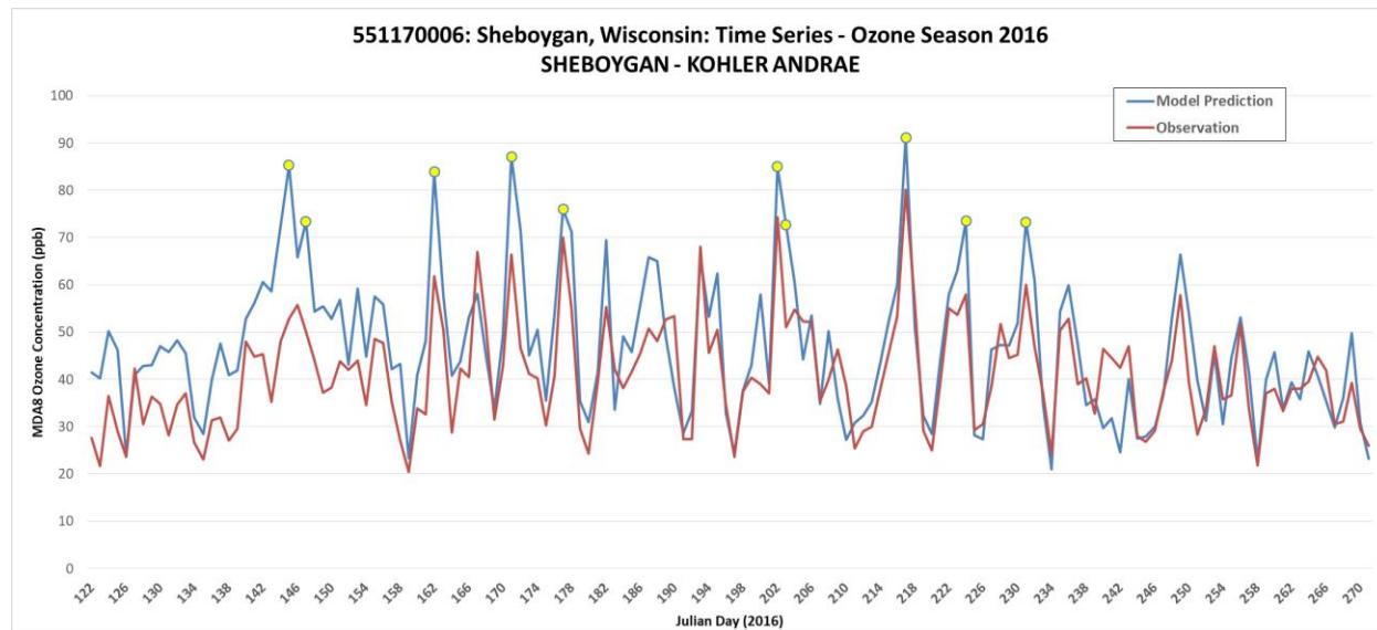
**Figure 80.** Time series of observed (red) and predicted 12km (blue) MDA8 ozone for May through September 2016 at site 551170006. Yellow dots indicate top modeled values.
