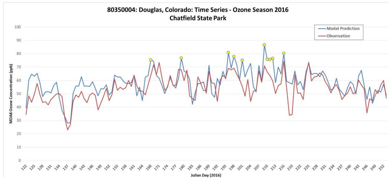
**Figure 112.** Time series of observed (red) and predicted 12km (blue) MDA8 ozone for May through September 2016 at site 80350004. Yellow dots indicate top modeled values.
