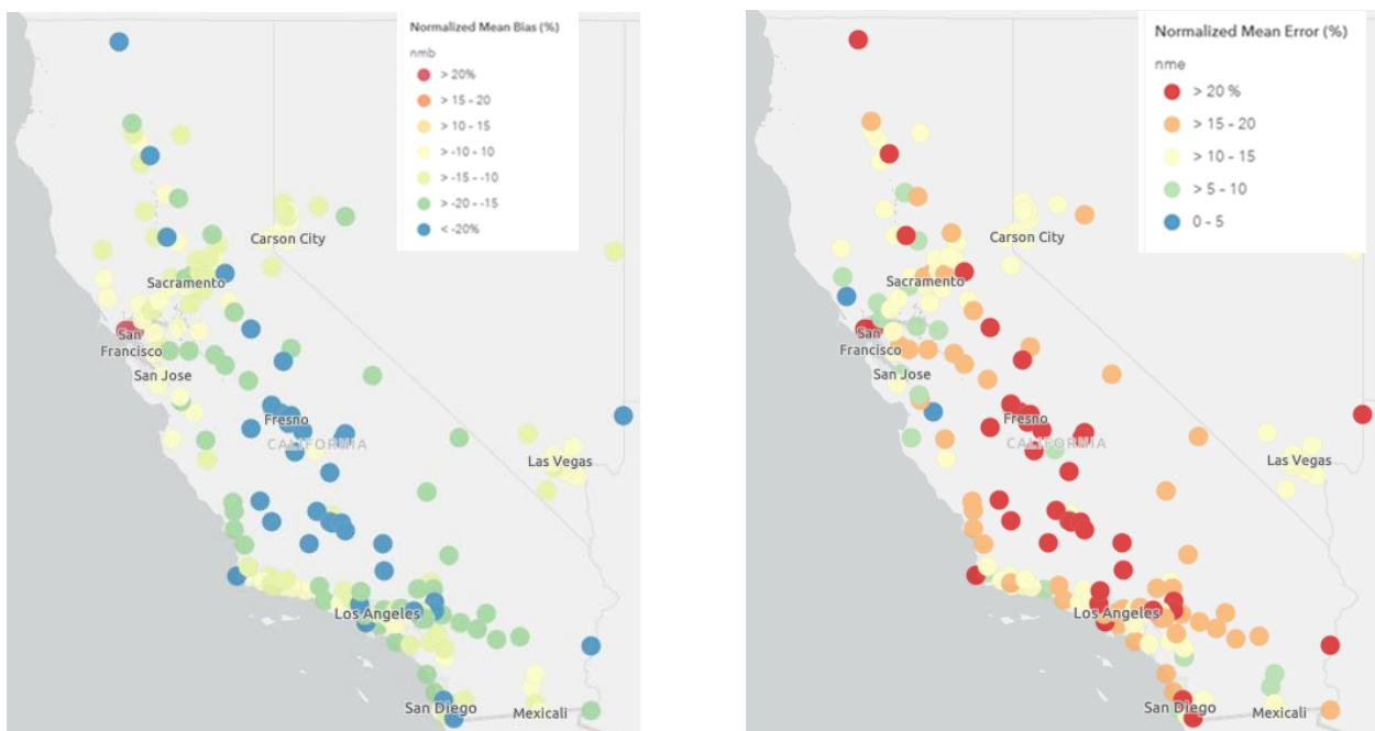
**Figure 45. Normalized Mean Bias (%) [left] and Normalized Mean Error (%) [right] of MDA8 ozone  $\geq 60$  ppb over the period May-September 2016 at AQS monitoring sites in West region.**
