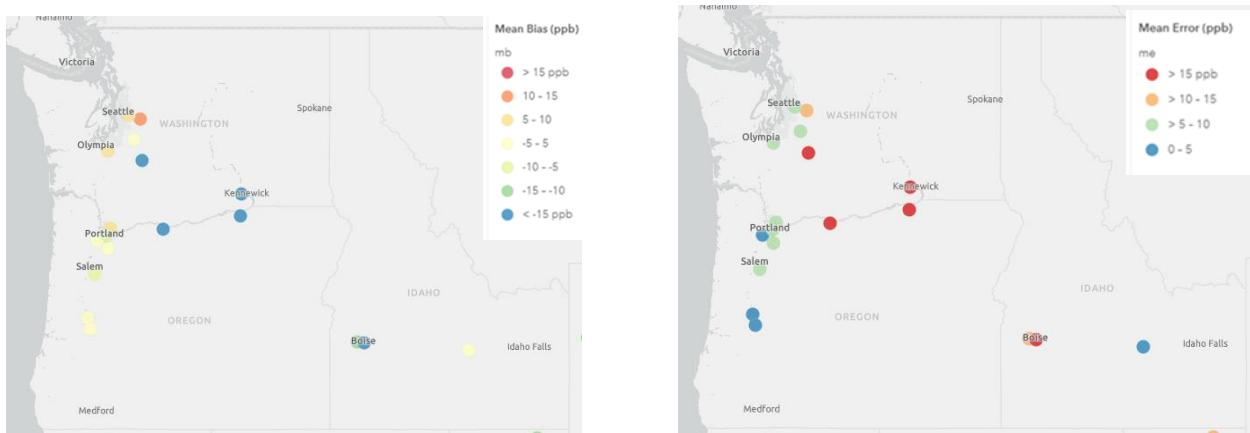
**Figure 24. Mean Bias (ppb) [left] and Mean Error (ppb) [right] of MDA8 ozone  $\geq 60$  ppb over the period May-September 2016 at AQS monitoring sites in Northwest region.**
