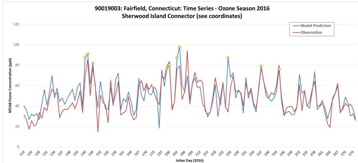
**Figure 84.** Time series of observed (red) and predicted 12km (blue) MDA8 ozone for May through September 2016 at site 90019003. Yellow dots indicate top modeled values.
