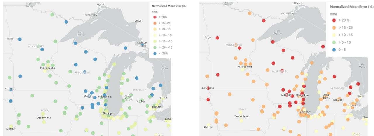
**Figure 15. Normalized Mean Bias (%) [left] and Normalized Mean Error (%) [right] of MDA8 ozone  $\geq 60$  ppb over the period May-September 2016 at AQS monitoring sites in in East-North-Central region.**
