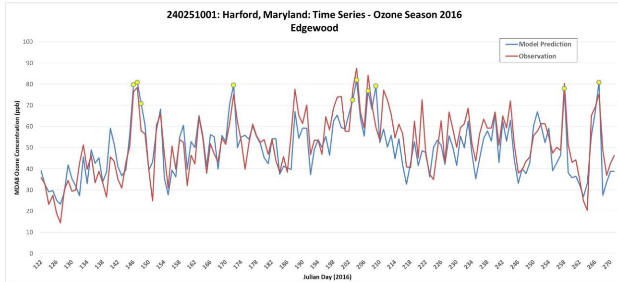
Figure 90. Time series of observed (red) and predicted 12km (blue) MDA8 ozone for May through September 2016 at site 240251001. Yellow dots indicate top modeled values.
