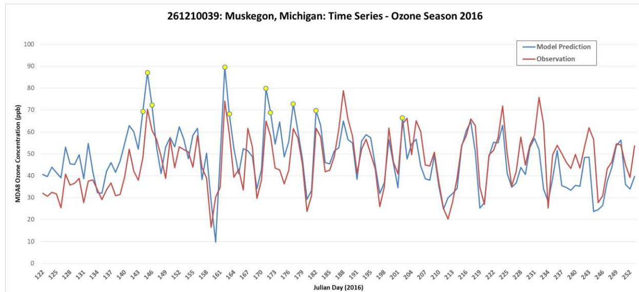
**Figure 78.** Time series of observed (red) and predicted 12km (blue) MDA8 ozone for May through September 2016 at site 261210039. Yellow dots indicate top modeled values.
