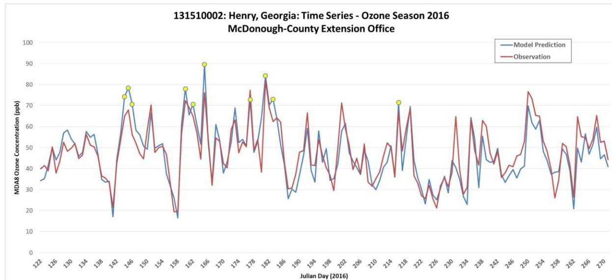
**Figure 108.** Time series of observed (red) and predicted 12km (blue) MDA8 ozone for May through September 2016 at site 131510002. Yellow dots indicate top modeled values.
