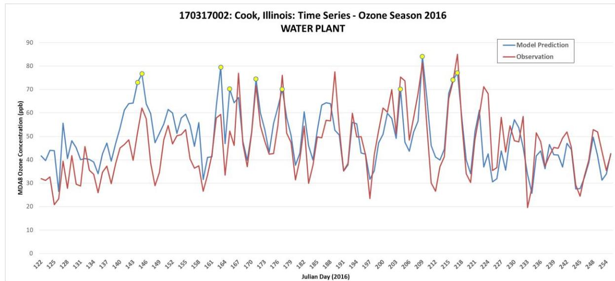
**Figure 72.** Time series of observed (red) and predicted 12km (blue) MDA8 ozone for May through September 2016 at site 170317002. Yellow dots indicate top modeled values.
