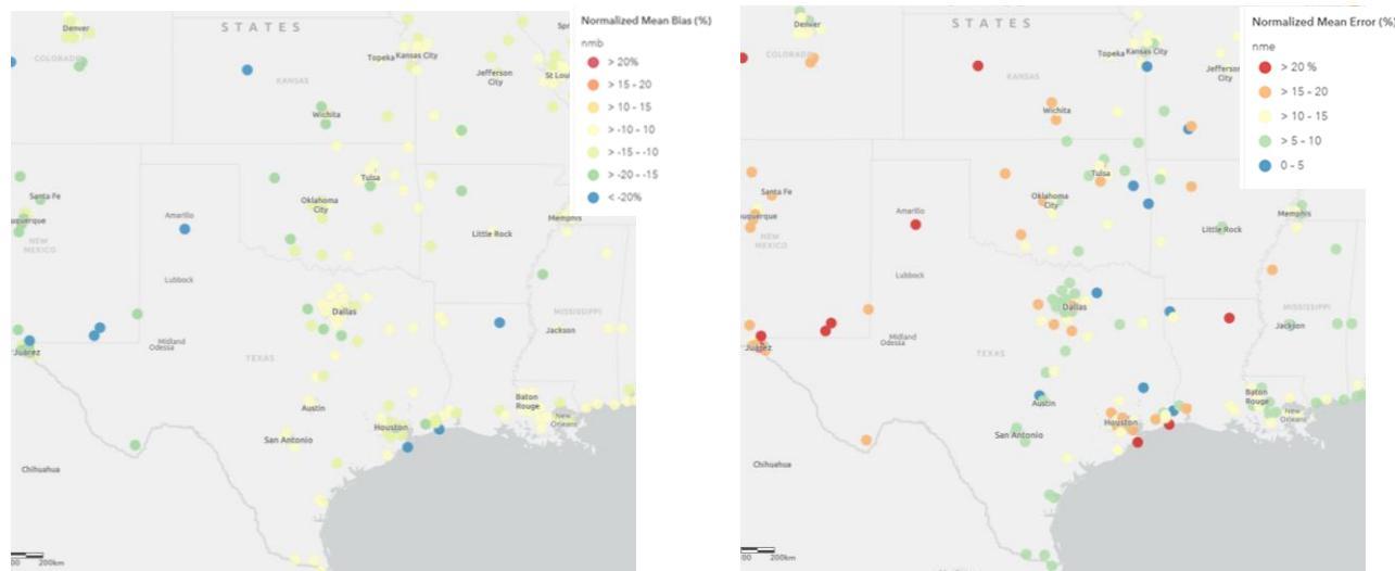
Figure 30. Normalized Mean Bias (%) [left] and Normalized Mean Error (%) [right] of MDA8 ozone  $\geq 60$  ppb over the period May-September 2016 at AQS monitoring sites in South region.
