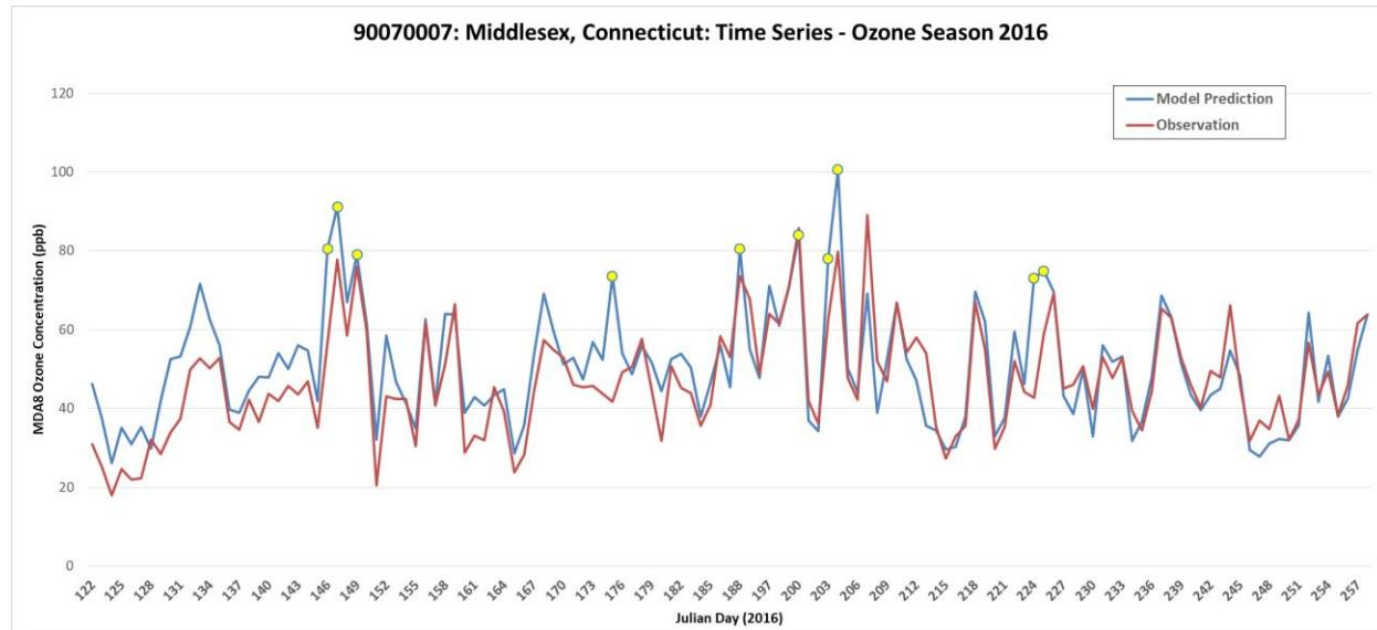
**Figure 86.** Time series of observed (red) and predicted 12km (blue) MDA8 ozone for May through September 2016 at site 90070007. Yellow dots indicate top modeled values.
