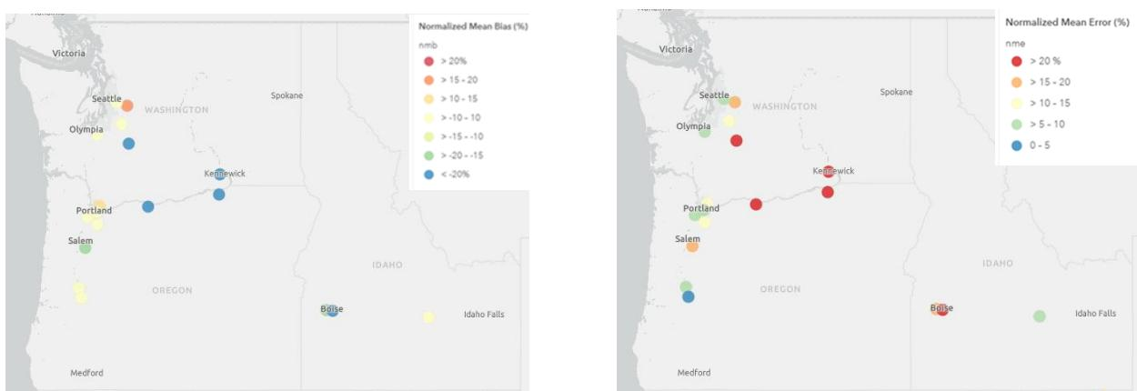
**Figure 25. Normalized Mean Bias (%) [left] and Normalized Mean Error (%) [right] of MDA8 ozone  $\geq 60$  ppb over the period May-September 2016 at AQS monitoring sites in Northwest region.**
