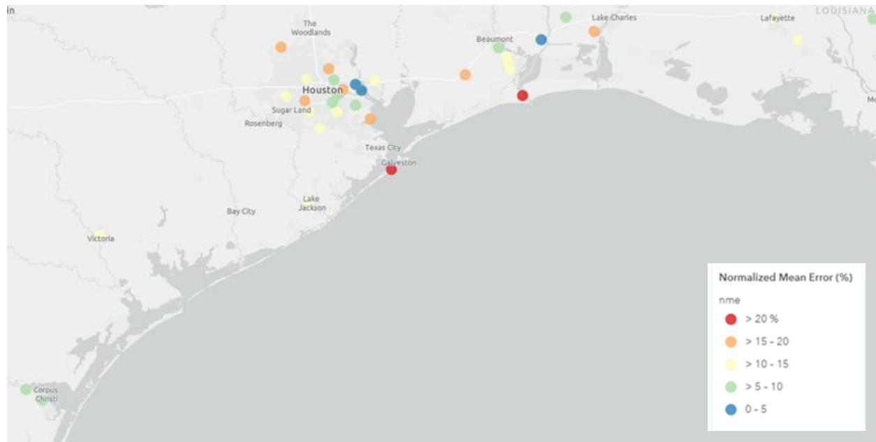
**Figure 58. Normalized Mean Error (%) of MDA8 ozone  $\geq 60$  ppb over the period May-September 2016 at AQS monitoring sites in Gulf Coast region.**
